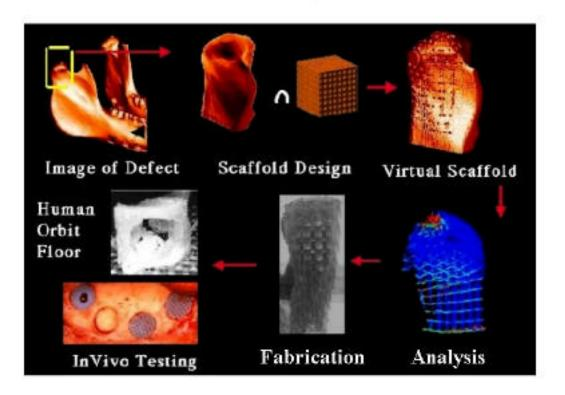
In addition to polygon models we have created, we can actually build physical replicas of Visible Human anatomy using solid free-form fabrication techniques. The orbit floor in the picture was built from patient CT data. Similar models have been built using VH data.
